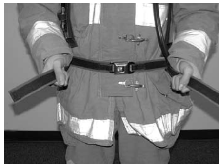
Figure 6. Tighten Waist Strap
